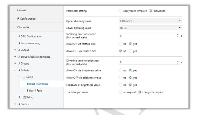
Fig 22: Ballast X Dimming Parameter Page Configuration
