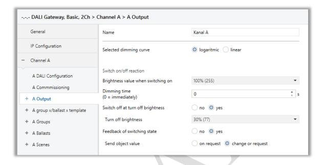
Fig 11: A Output Configuration
