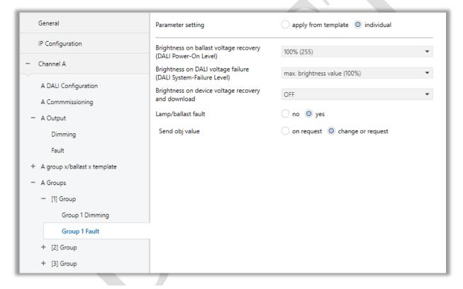
Fig 20: Group X Fault Parameter Page Configuration
