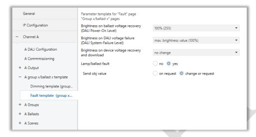
Fig 16 : Fault Template (Group x / Ballast x) Configuration
