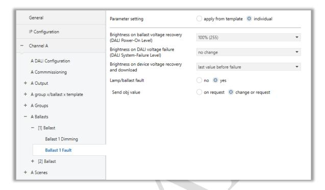
Fig 23: Ballast X Fault Parameter Page Configuration
