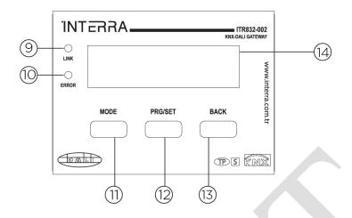
Figure 3: Buttons & LCD Features of KNX-DALI Gateway
