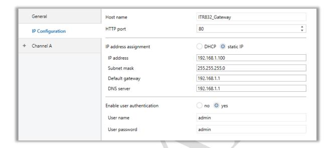
Fig 8: IP Configuration Parameter Page
