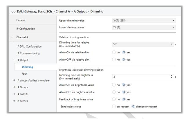
Fig 12: Dimming Function Configuration
