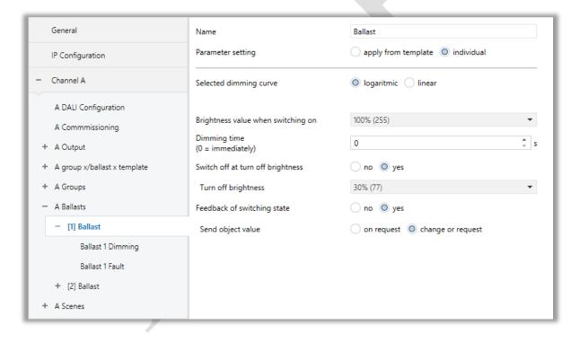
Fig 22: [x] Ballast Parameter Page Configuration
