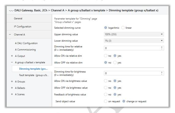
Fig 15: Dimming Template (Group x / Ballast x) Configuration
