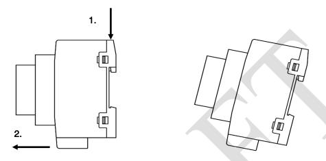
Figure 6 : Demounting method of KNX-DALI Gateway
